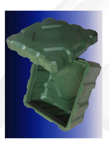
When manufacturing rotomoulded products, it is possible to include ribs of various types to reinforce the points subjected to particular stress. The recommended depth is about four times the material thickness, while the width should be about five times the material thickness. These parameters are generally applicable and can vary according to the geometry of the product and to its condition of use.
